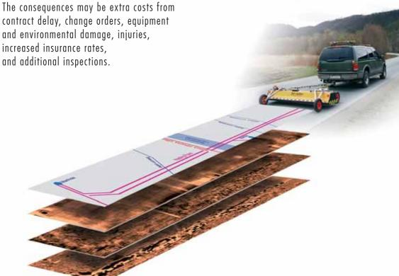
The 3d-Radar GPR provides 3-dimensional images of the subsurface down to 2 meters and gives the user a unique opportunity to plan and conduct efficient excavation in urban areas. The system allows scanning of large areas and mapping of the underground infrastructure and other obstacles below the pavement.
